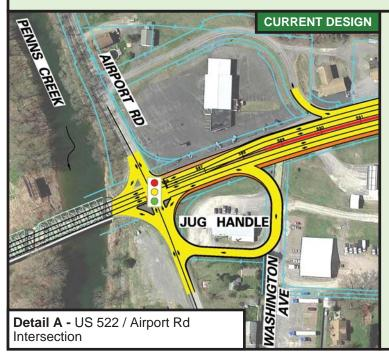
To ensure efficient traffic flow in the future, the existing two lane section of US 522 southbound will be extended from the interchange through the Airport Road intersection and carried across the existing truss bridge over Penns Creek toward Selinsgrove.
