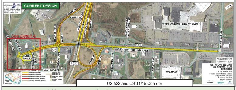
At the interchange of CSVT, US 522 and US 11/15, ramps have been reconfigured to improve geometry and operations. Most notably, the existing northbound off ramp geometry has been improved to flatten the curve as the ramp merges with US 11/15 northbound. Two northbound US 522 lanes are needed through the interchange to accommodate projected future traffic volumes. Therefore, a third lane on US 11/15 northbound has been added to the design, extending from the interchange to Roosevelt Avenue.
